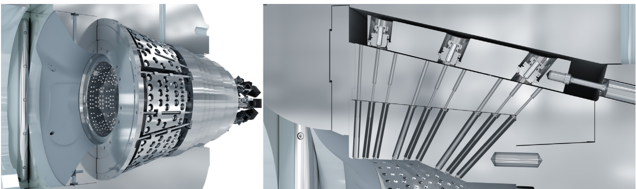
Illustration of the radiation unit with the moveable sectors (left) and the source collimation system (right).
