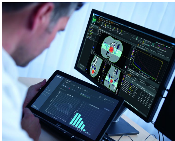
Validation of a prostate treatment plan with myQA iON. Irradiation Log based patient QA using the Spot Map Analysis function.
