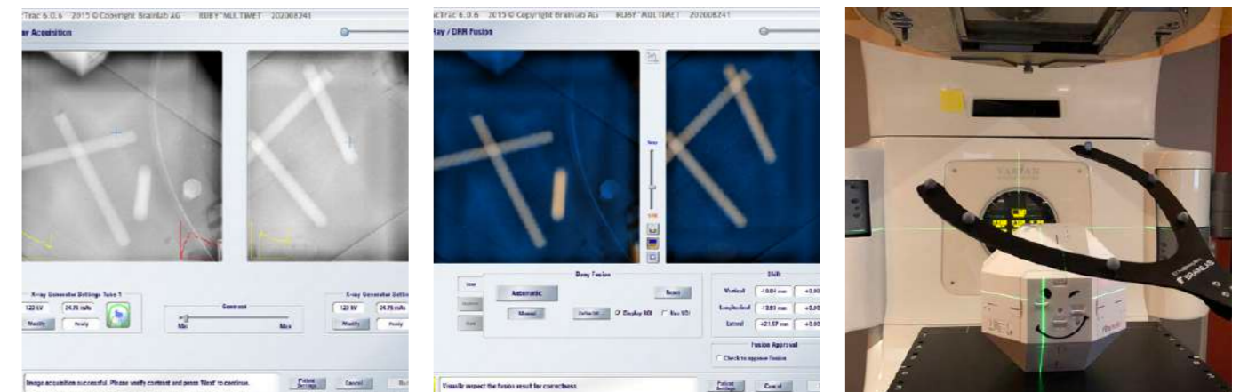
Figure 20: kV image registration of the System QA MultiMet insert. Left: kV images before image registration. Center: After image registration. Right: RUBY phantom with System QA MultiMet insert and Brainlab frame.
