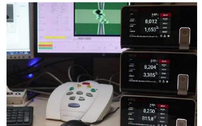
Figure 21: Simultaneous dose measurement in the System QA MultiMet insert using three PinPoint 3D ionization chambers and three UNIDOS Tango systems
