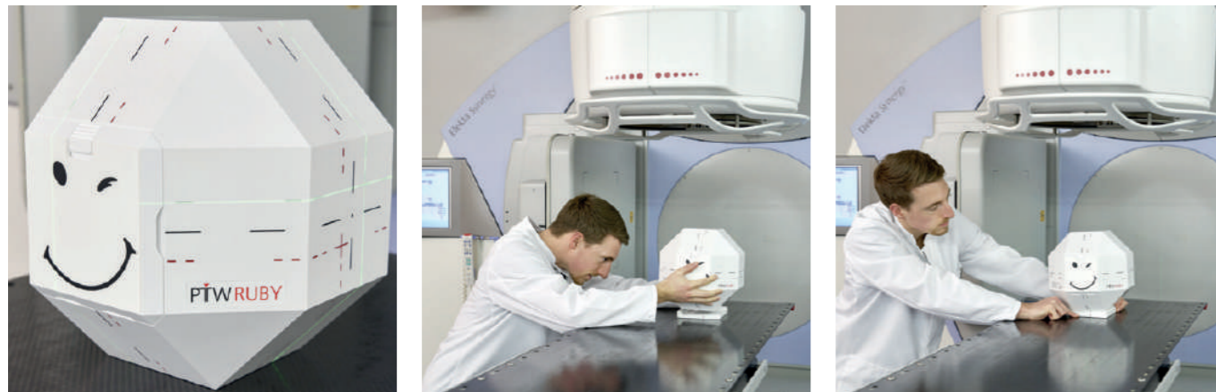
Figure 2: Left: RUBY aligned using the grey line with translational misalignment. Center and right: Combination of the tilting base and alignment according to the red line for translational and rotational misalignment.
