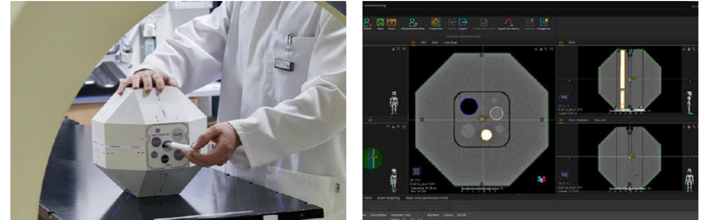
Figure 11: Left: Planning CT of RUBY. The detector cavity is filled with a homogenous plug. Right: CT dataset of the System QA insert.
